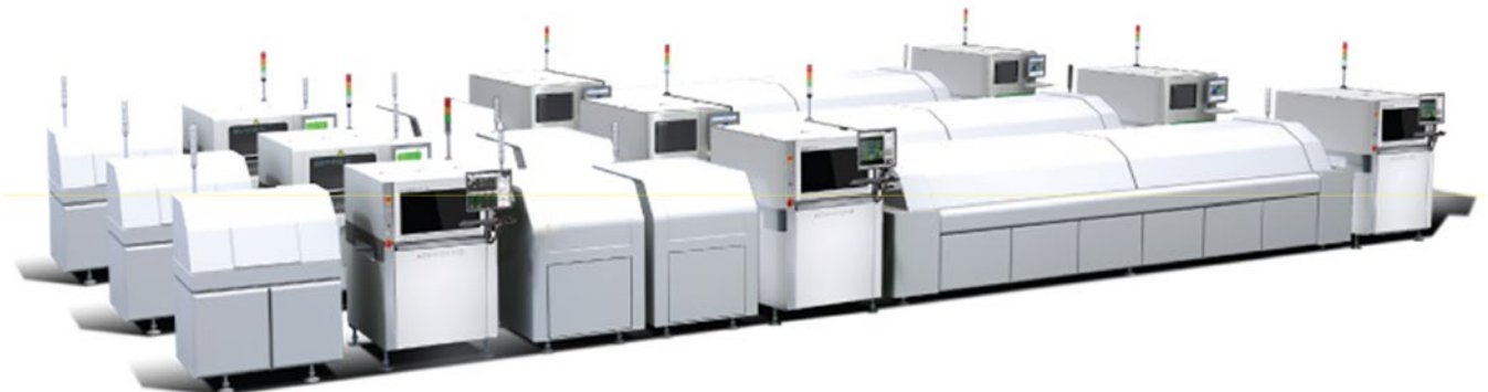
Figure 2: Theoretical SMT lines using APC active feedback between solder paste printer, SPI, component mounter, and AOI systems.
